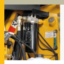
Vertical filters allow quick, no-spill changes. Engine, hydraulics, and transmission utilize a common oil, further simplifying service.
