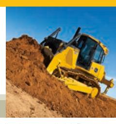
No need to cross-steer or ride a brake. These dozers steer the same and maintain their preset speed whether working on level ground or a 2-to-1 slope.
