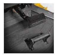
Choose the decelerator function that's right for the job. Slow both ground speed and engine rpm, or ground speed only to help maintain traction without affecting engine power and hydraulic response. Fully depressing the pedal applies the brakes.
