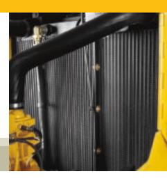
No stacked coolers in these crawlers. Side-by-side cores with wide fin spacing reduce clogging and are easy to clean.
