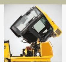
Operator station tilts a full 70 degrees in only minutes, for wide-open access to internal components. Unlike other crawlers, there's no need to disconnect linkages, hydraulics, or wiring.
